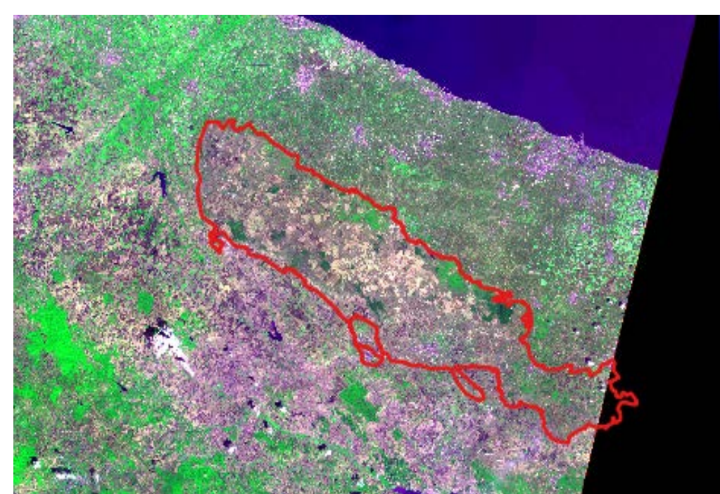
T 2 data: Sentinel-2 image August 7, 2016 False Color: R=B3, G=B4, B=B2 20 meters – VIS/NIR/SWIR
